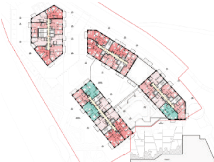
09.11 Typical floor plan — apartment layouts reworked around the revised shafts. / PLAN
