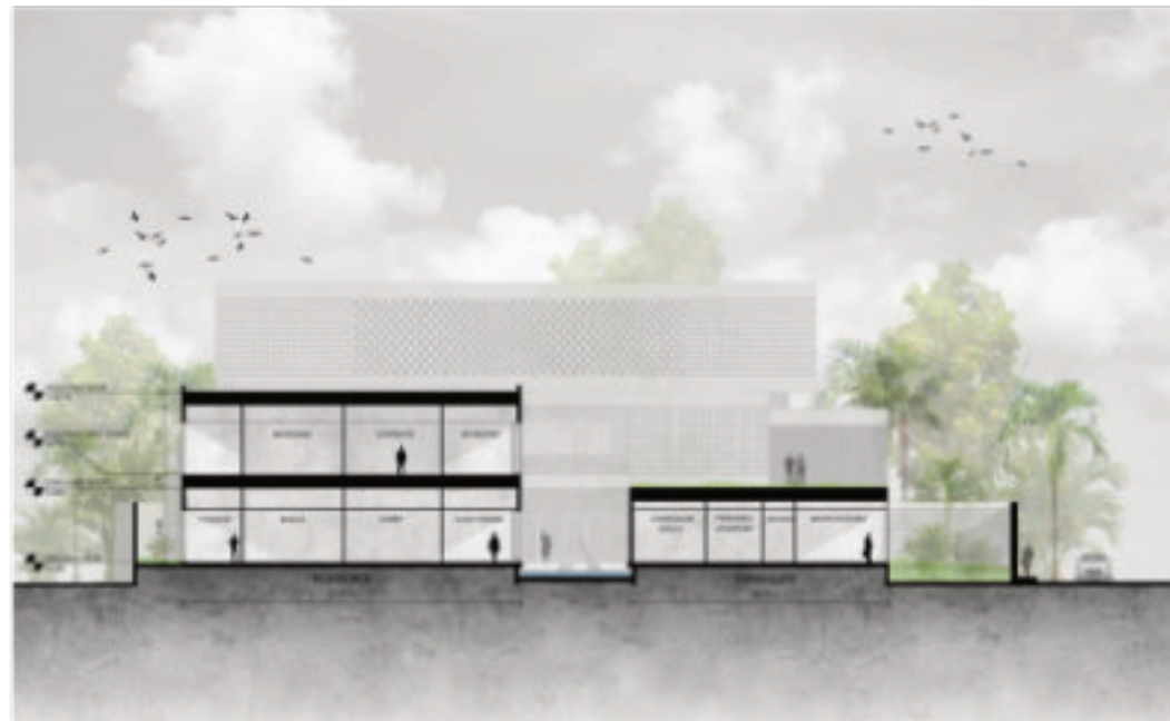
08.12 Section through the residence and consulate — the roof garden recovering the green space. / SECTION
