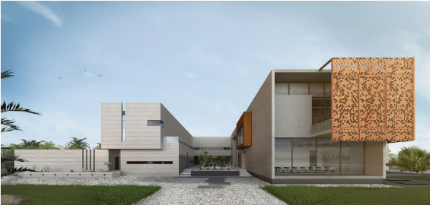
04.1 Contemporary mashrabiya screens on the garden elevation — the curtain-wall panel system controlling privacy and solar exposure. / EXTERNAL VIS.
